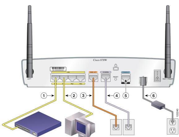
Figure 1-9 Typical Installation of a Cisco 878 Router
